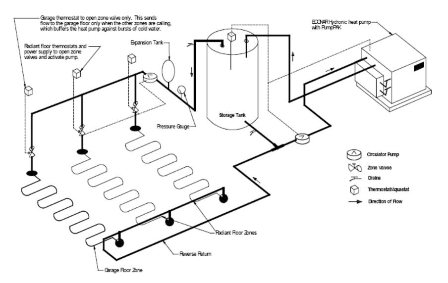
Note – Always use copper pipe on the hydronic side.
