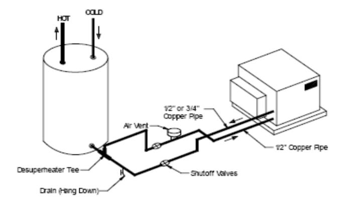
Note – Always use copper pipe. Check local codes and use proper plumbing procedures.
