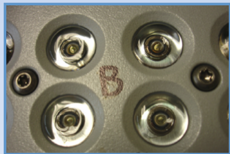
Light Bar (after 54 weeks of temperature cycling)
